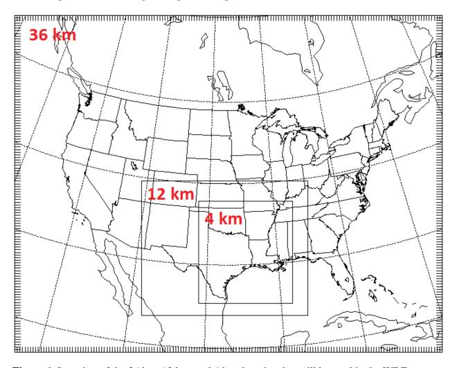
**Figure 1.** Location of the 36 km, 12 km, and 4 km domains that will be used in the WRF modeling. The CMAQ modeling domains will be slightly smaller than the WRF modeling domains (grid cells close to the horizontal edge of the WRF domains will not be included in the CMAQ domains).
